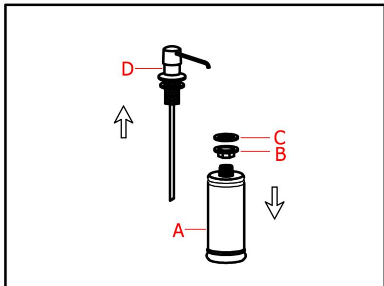
1. Unscrew the bottle (A), lock nut (B) and rubber washer (C) from the pump assembly (D).
