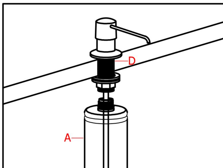
4. Thread the bottle (A) into the pump assembly (D) until secure. (**Note:** Do not overtighten.)
