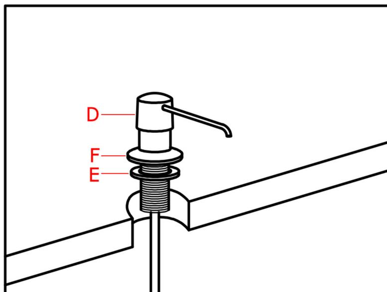
2. Insert the pump assembly (D) through the mounting hole. Make sure the rubber washer (E) is fitted into the pump base (F).
