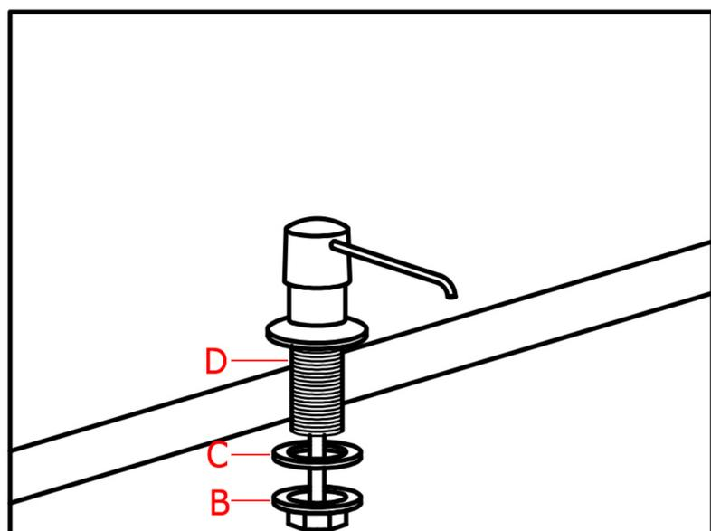
3. Underneath the countertop, slide rubber washer (C) and lock nut (B) onto the pump assembly (D). Position the pump assembly (D) correctly, fixing the lock nut (B) tightly.
